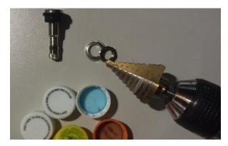
After drilling the hole use the small pocket knife to trim off excess material and part of the gasket if its still attached.
